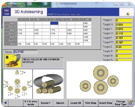
5- Program Calculated by CNC
