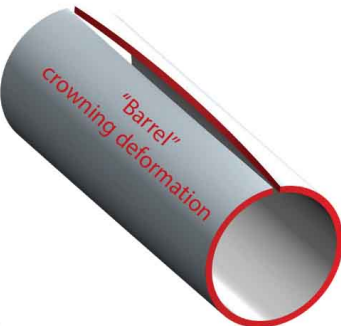
Bending thickness is thicker than roll crowning
