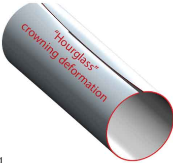
Bending thickness is thinner than roll crowning
